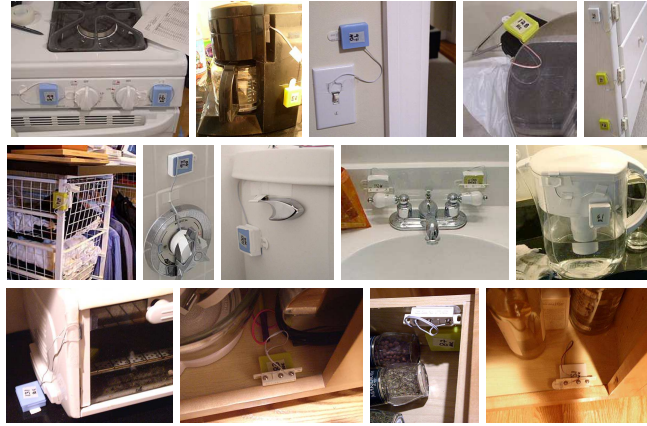
Fig. 2. Examples of some of the 77 sensors that were installed in the home of the first subject. The sensors and data collection boards were literally taped to objects and surfaces for the duration of the data collection period.
