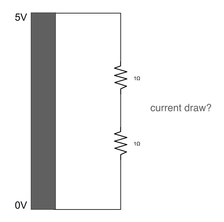
battery capacity = 110mAh 110 mA for 1 hour 220 mA for 1/2 hour 2.5A for ??
