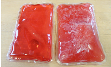
Sodium acetate in room temperature. Super cooled liquid state (left) and solid state (right)
