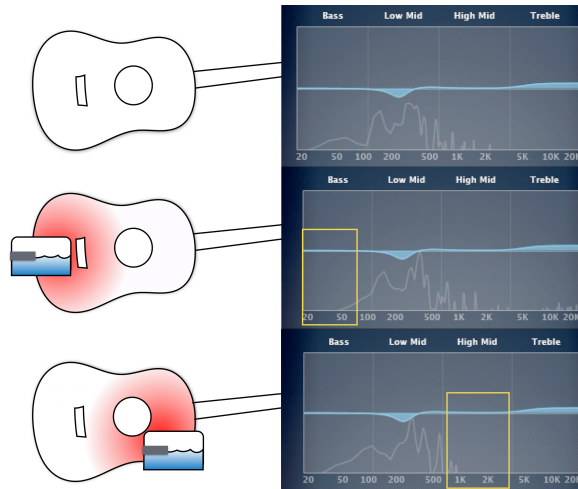
Figure 4. Using the L-Shift concept, we explored how weight-change impacts sound.
