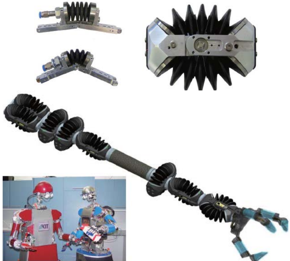
Fig. 25: Fluidic Arm (large picture) and Humanoid Robot ARMAR III with Fluidic Robotic Hands FRH 4/5 (small picture)
