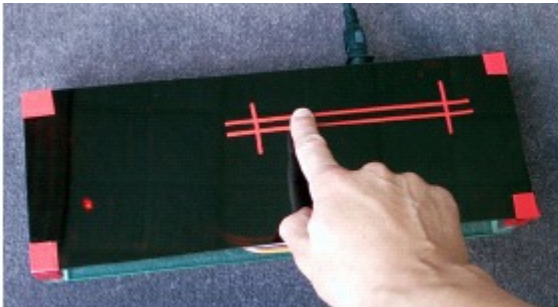
Figure 9: Slider Demo - Glass Cermaic removed to Show Electrodes and Circuitry
