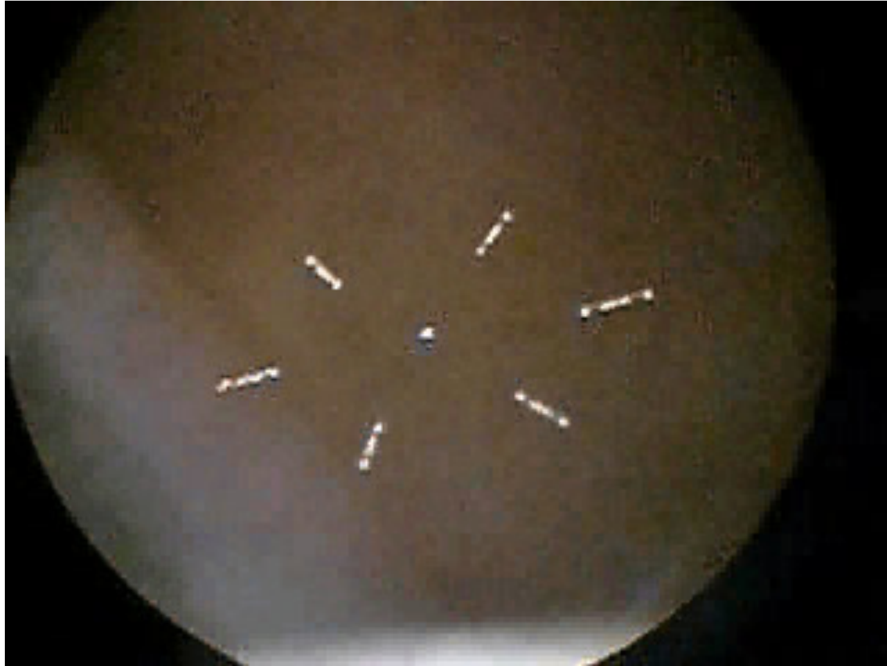
Actual image of oscillating particle clusters in trap
